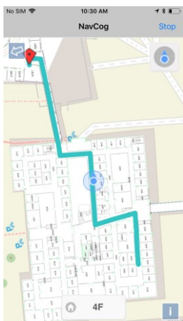
Figure 3. NavCog3 [14] is an open source smartphone-based indoor navigation system for people with visual impairments. An auditory interface provides turn-by-turn directions and immediate feedback when incorrect orientation is detected. Image courtesy NavCog ( http://www.cs.cmu.edu/~NavCog/navcog.html ).
